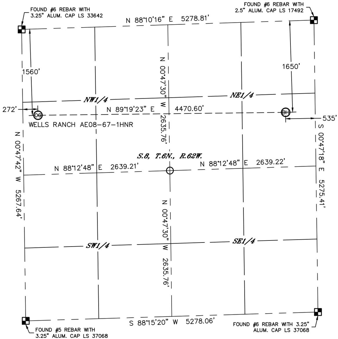
In accordance with a request from Sean Casper with Noble Energy Inc. Lat40°, Inc. has determined the surface location of the WELLS RANCH AE08-67-1HNR to be 1560' from the NORTH line and 272' from the WEST line and the bottom hole to be 1650' from the NORTH line and 535' from the EAST line as measured at right angles from the section lines of Section 8, Township 6 North, Range 62 West of the Sixth Principal Meridian, County of Weld, State of Colorado.
