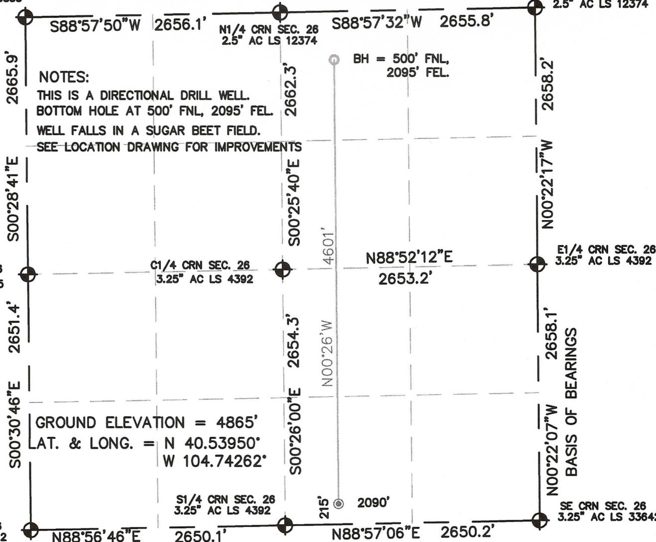
I HEREBY STATE TO PERTOLEUM DEV. CORP. THAT THE SURFACE LOCATION OF THE WELL LEFFLER 34-26H IS LOCATED 215' FSL & 2090' FEL, SEC. 26, T7N, R66W, 6PM.
