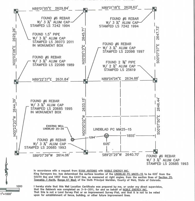
1) Bearings shown are Grid Bearings of the Colorado State Plane Coordinate System, North Zone, North American Datum 1983/2007. The lineal dimensions as contained herein are based upon the "U.S. Survey Foot."
