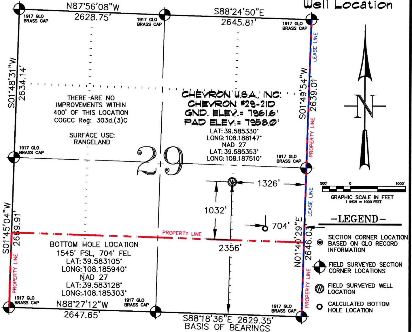
**THIS WELL LOCATION PLAT WAS PREPARED FOR BERRY PETROLEUM COMPANY, TO LOCATE THE CHEVRON #29-21D WELL, 2356 FEET FROM THE SOUTH LINE AND 1326 FEET FROM THE EAST LINE IN THE NW1/4 SE1/4 OF SECTION 29, T. 5 S., R. 96 W. OF THE 6TH P.M. GARFIELD COUNTY, COLORADO.**
