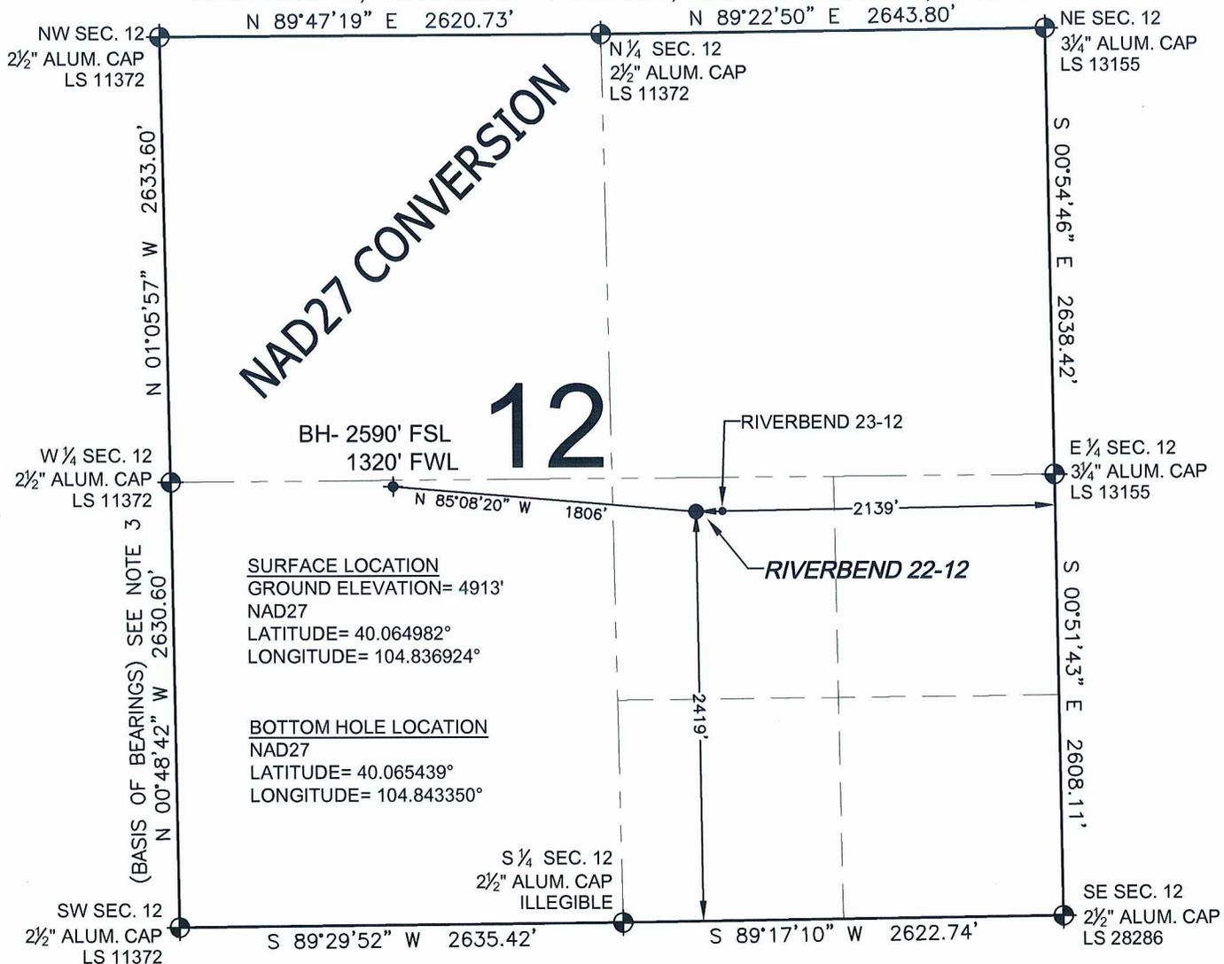
WELL **RIVERBEND 22-12** TO BE LOCATED 2419' FSL AND 2139' FEL, SECTION 12, T1N, R67W OF THE 6th P.M.
