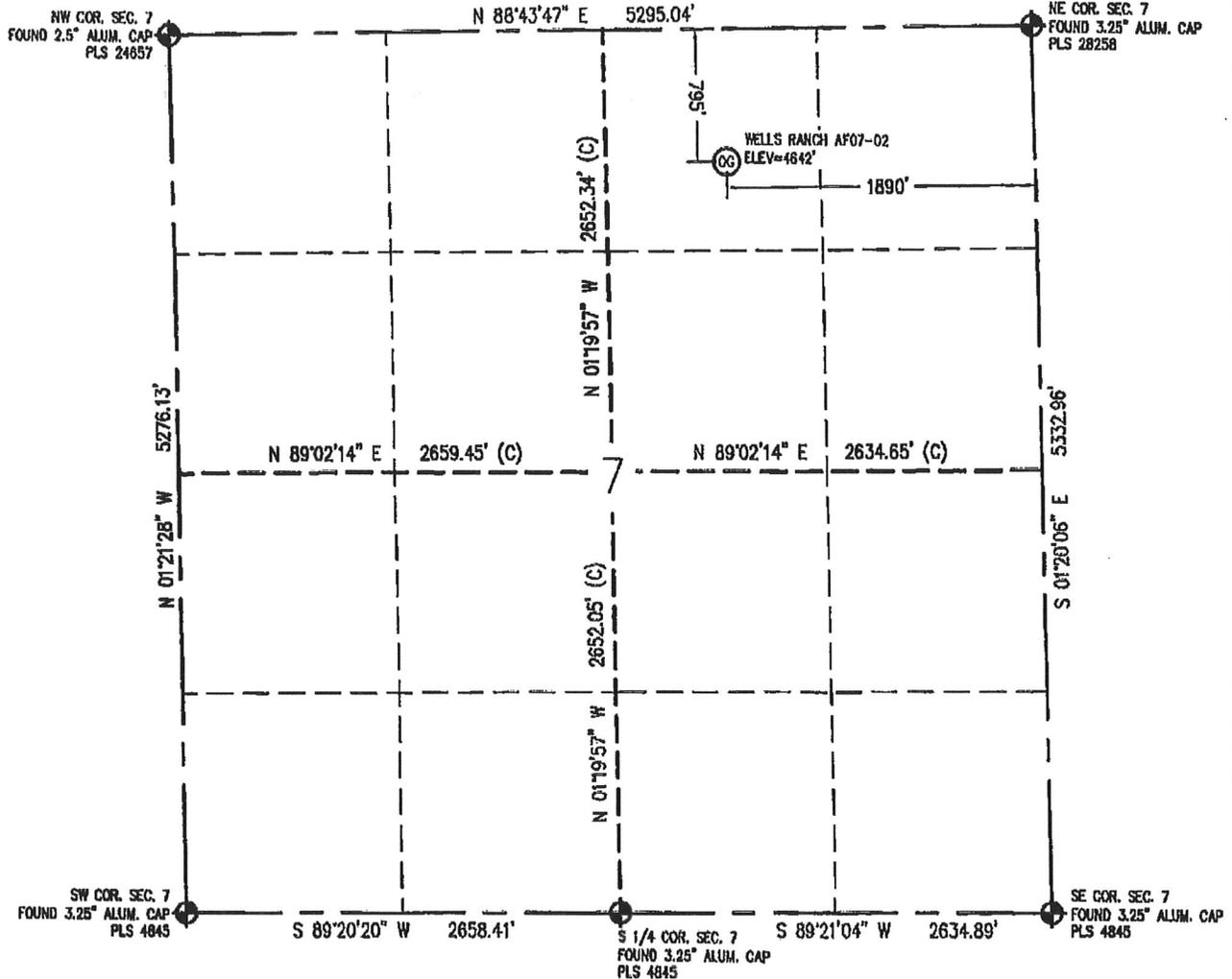
IN ACCORDANCE WITH A REQUEST FROM SEAN CASPER - NOBLE ENERGY, BASELINE ENGINEERING CORP. HAS DETERMINED THE LOCATION OF THE WELLS RANCH AF07-02 TO BE 795' FNL AND 1890' FEL, AS MEASURED AT NINETY (90) DEGREES FROM THE SECTION LINE OF SECTION 7, TOWNSHIP 5 NORTH, RANGE 62 WEST, 6TH PRINCIPAL MERIDIAN, WELD COUNTY, COLORADO.
