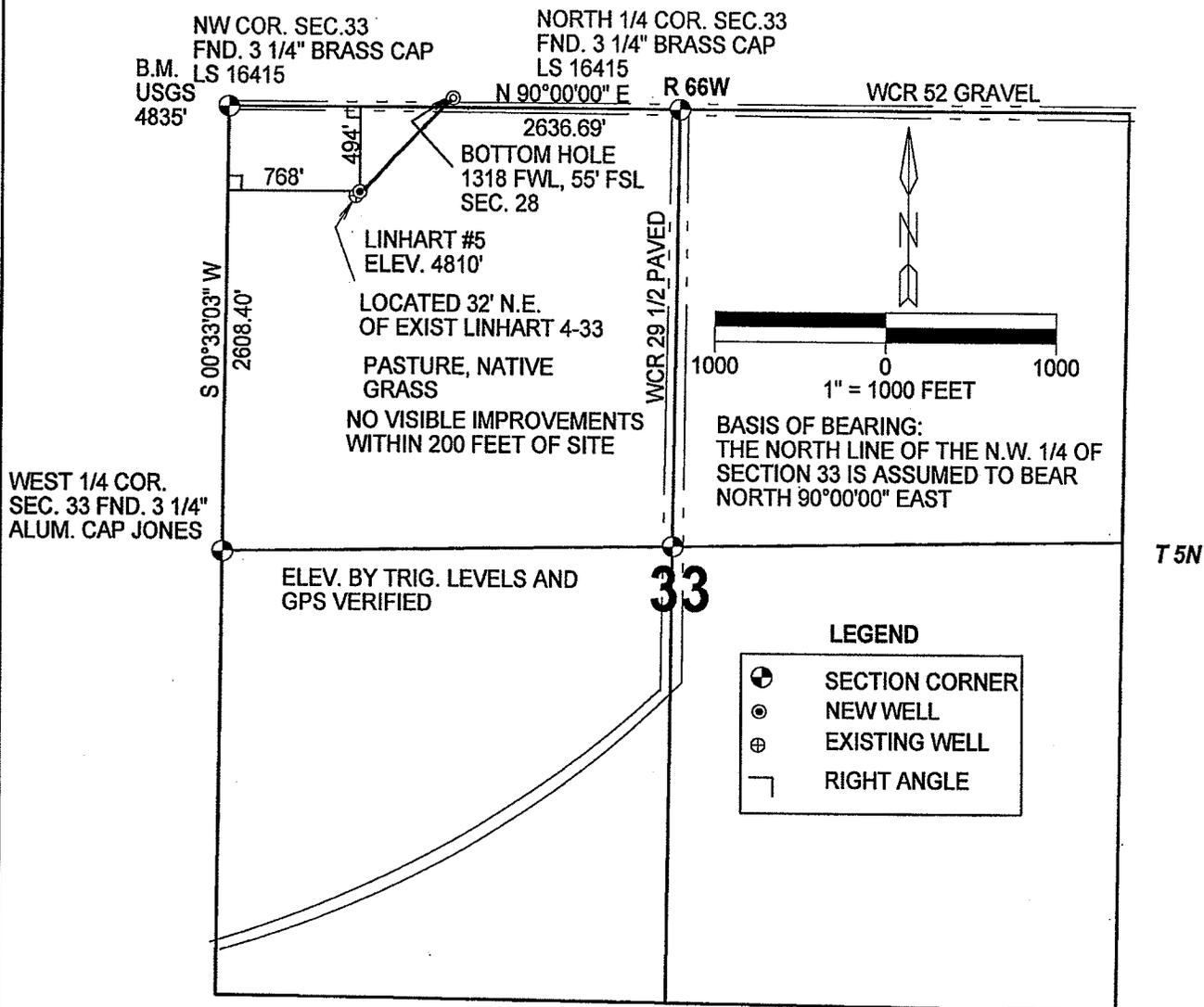
IN ACCORDANCE WITH A REQUEST FROM MERIT ENERGY COMPANY, THE UNDERSIGNED HAS DETERMINED THE LOCATION OF THE LINHART NUMBER 5 WELL TO BE 768' FWL AND 494' FNL, SECTION 33, TOWNSHIP 5 NORTH, RANGE 66 WEST OF THE 6TH PRINCIPAL MERIDIAN, WELD COUNTY, COLORADO. FIELD SURVEY DATE: MARCH 15, 2007
