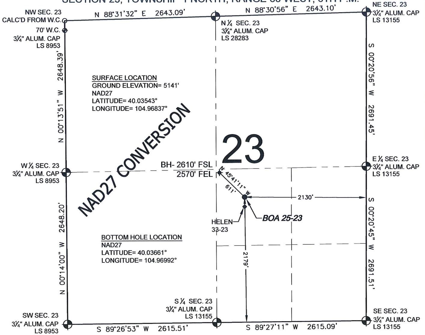
WELL **BOA 25-23** TO BE LOCATED 2179' FSL AND 2130' FEL, SECTION 23, T1N, R68W OF THE 6th P.M.
