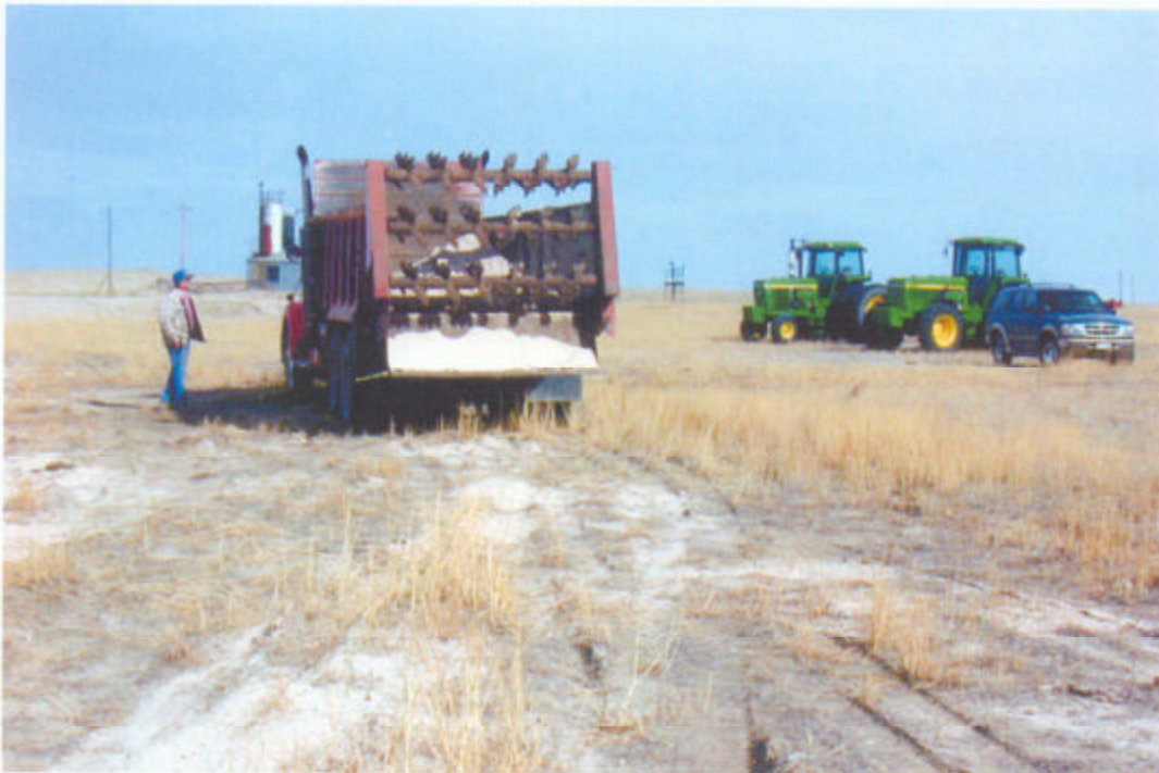
02 – Manure spreader used to distribute gypsum.
