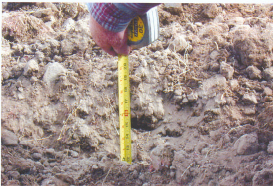
07 – Depth of sub-soiler penetration
