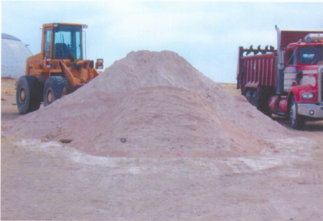
01 – Agricultural grade Gypsum delivered in bulk to the project site. CASE front-end loader used to load and weigh (3 tons/bucket) gypsum. Manure spreader to right used to distribute gypsum.
