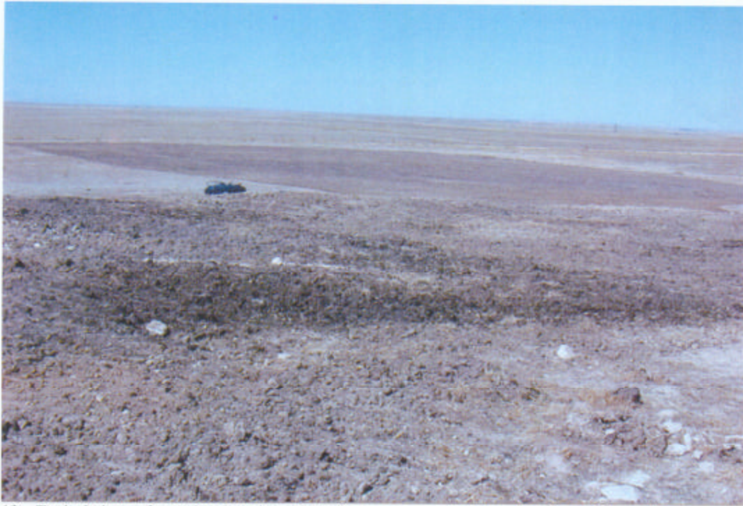
13 – Typical photo of completed work product after gypsum application, chiseling, sulfur application and disking. Area 4 looking northwest.
