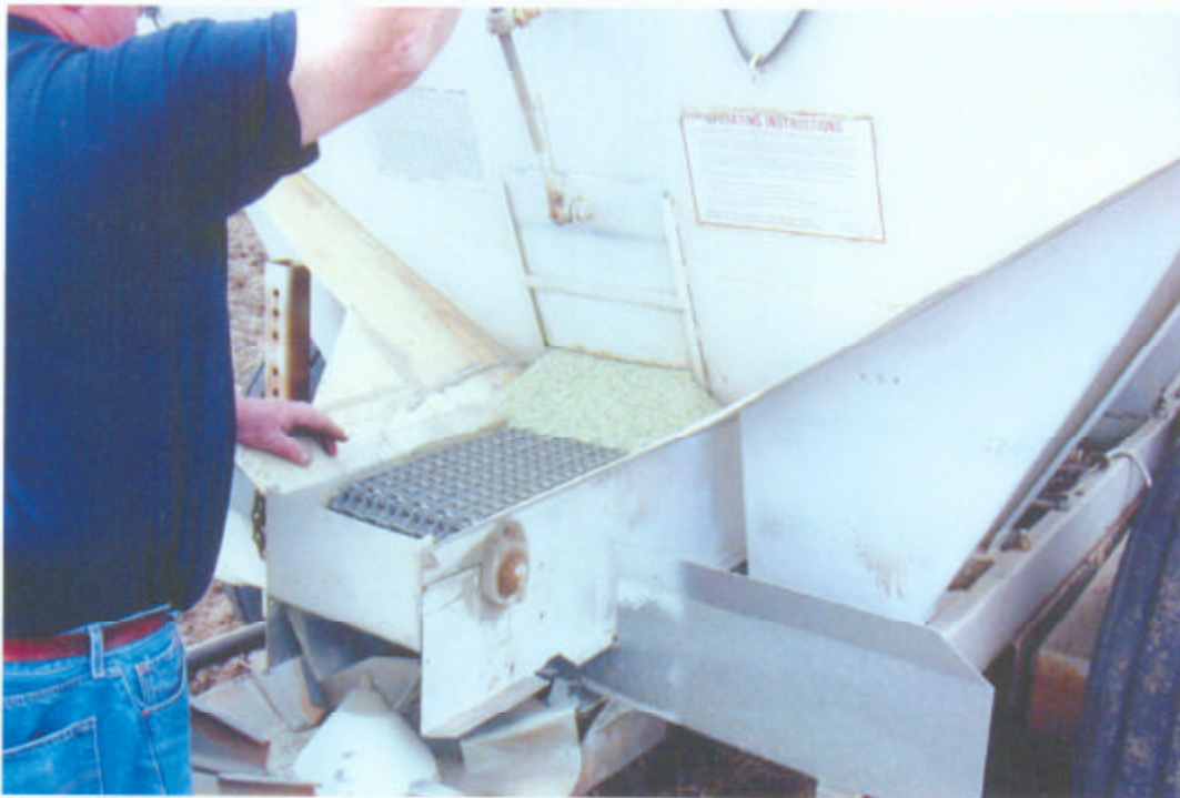
09 – Dry fertilizer spreader showing adjustable gate and rotary spreader.
