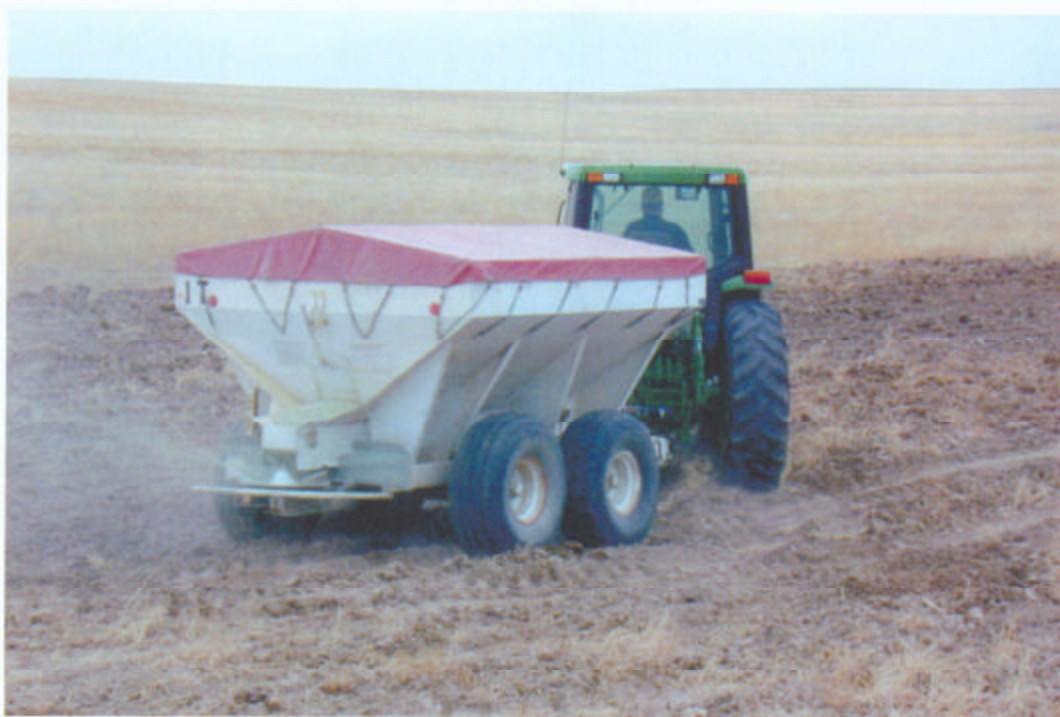
08 – Dry fertilizer spreader used to distribute sulfur.
